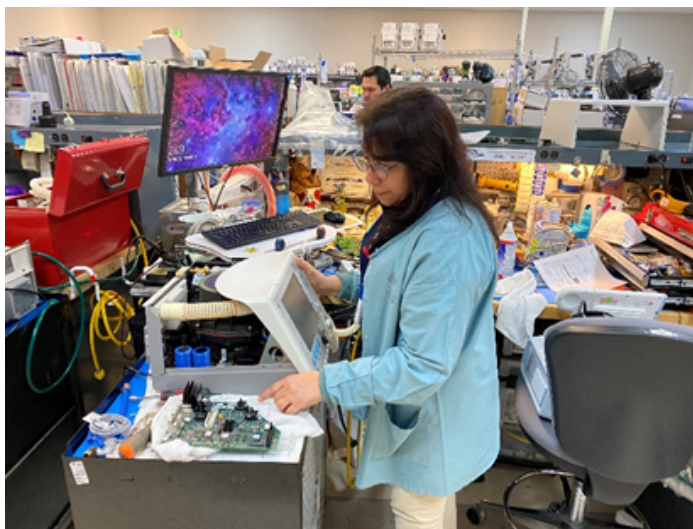
FIGURE. Engineering technician, Rocky, perform the final test on a ventilator before placing her signature on the tag that states – PATIENT READY.
