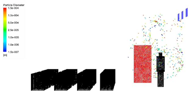
FIGURE 15. Particle distribution 10 s after coughing with side wall ventilation at 5 m/s.
