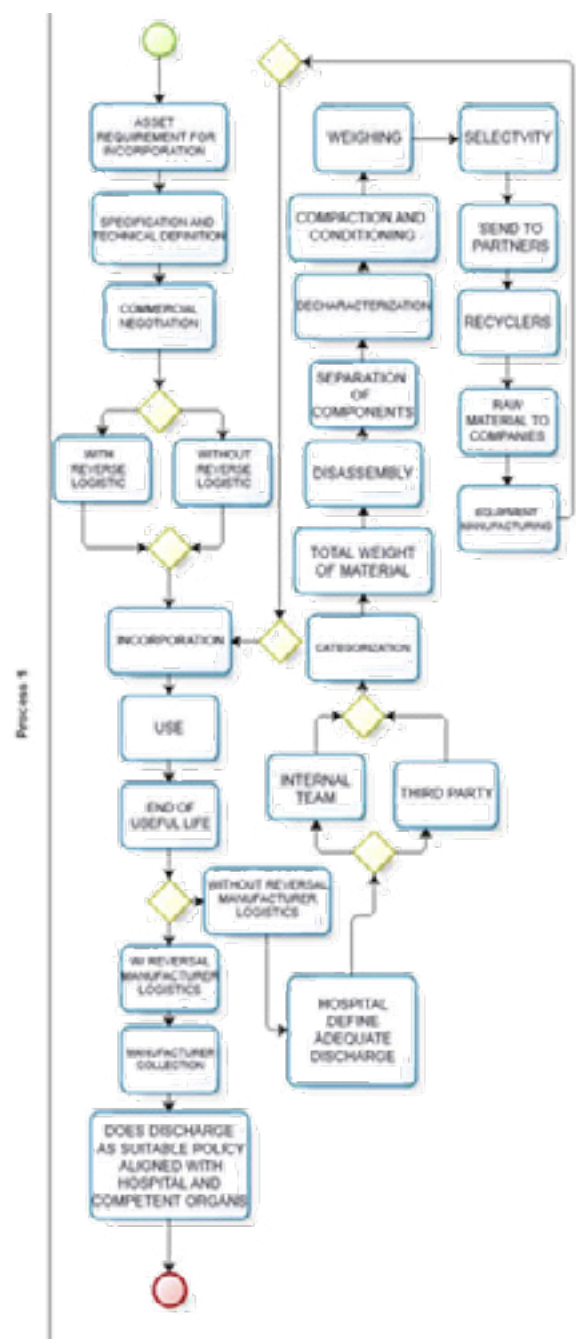
FIGURE 2. Proposed flow for discarding hospital electric and electronic equipment. Adapted from Meta-recycling. 1
