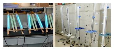
This is the disinfection method recommended by the prevention and control guidelines issued by the National Health and Safety Commission. Engineers carried out ultraviolet intensity testing in strict accordance with medical ultraviolet disinfection requirements and formulated usage specifications to more comprehensively ensure the protection and safety of patients, family members, and medical personnel.
