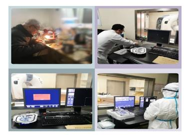
With the aim of not affecting the function of the CT equipment, the rack control panel was moved to the external operation room so that the operators could safely position themselves outside the CT room and avoid close contact with patients. This greatly reduced the risk of infection.
