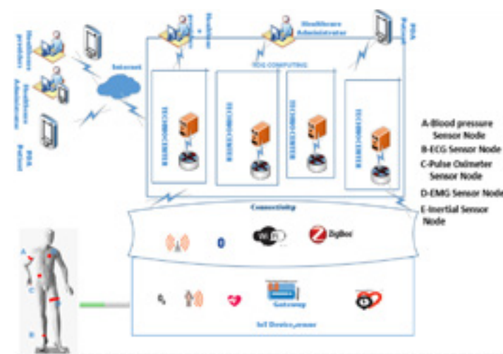
FIGURE 1. IoT architecture of an integrated patient monitoring network.
