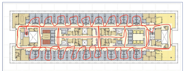
FIGURE 2. Example of marked up hospital floor plan, highlighting all places where patients will be monitored
