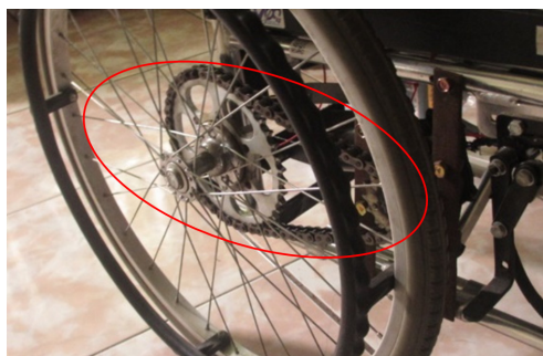
FIGURE 2. The chain used to connect the wiper and back wheel.
