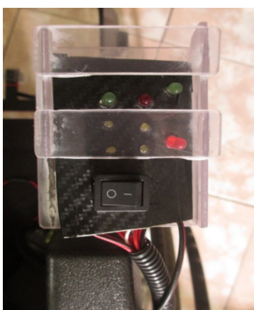
FIGURE 5. LED Indicators placed on the right armrest.
