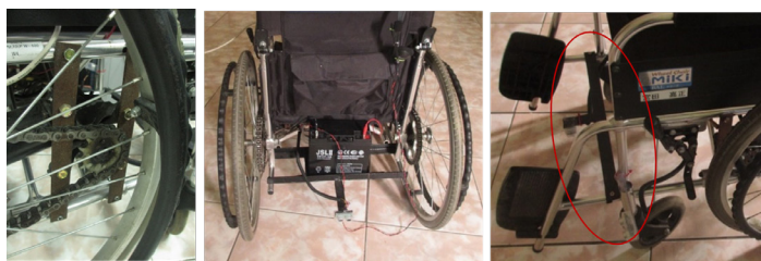
FIGURE 6. Flat bar attachment for wiper motors, battery, and ultrasonic sensor.
