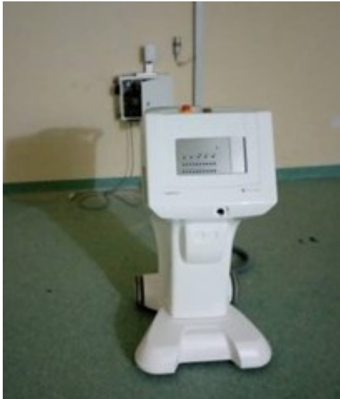
FIGURE 1. A 25-channel Saginova HDR afterloader brachytherapy unit installed by the local engineer.
